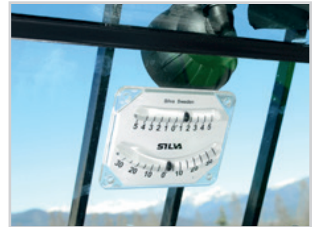
Lateral and longitudinal level indicators fitted to the windscreen and and RHS glass
