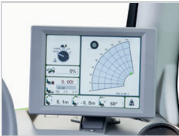
Merlo CDC (Dynamic Load Control) rated capacity limiter
