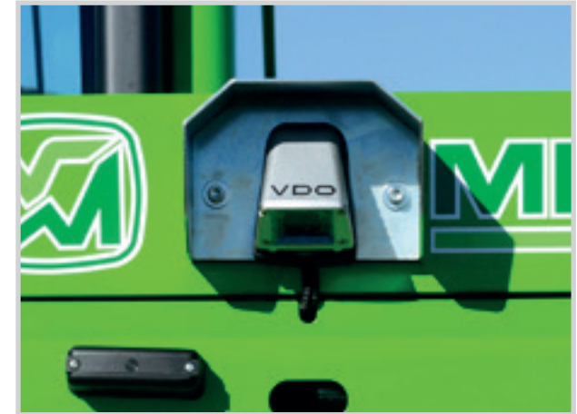
Rear camera starts automatically when engaging the reverse shuttle.
